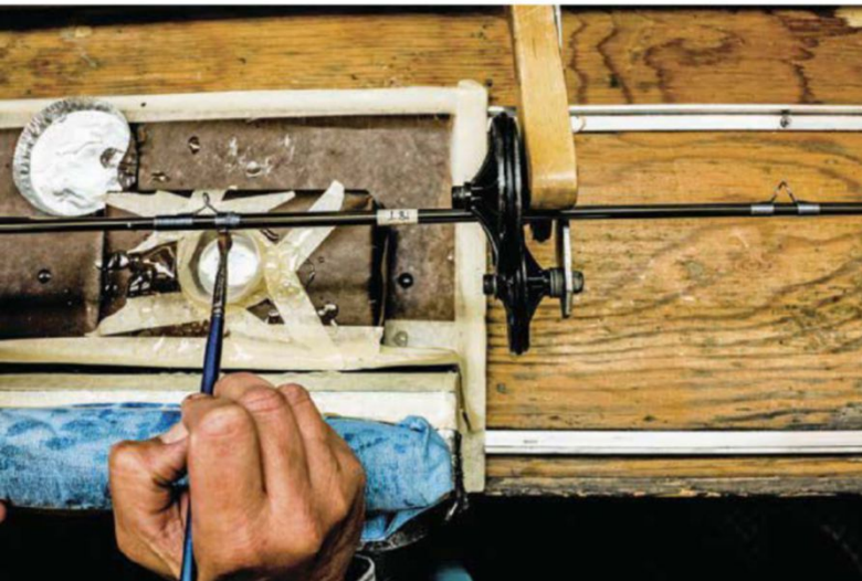
A worker seals the eyelets that guide the line along the rod
